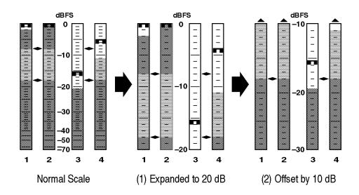
Figure 17: Creating a custom meter scale
